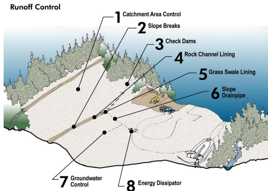
Figure 7.3: Surface Runoff Control
