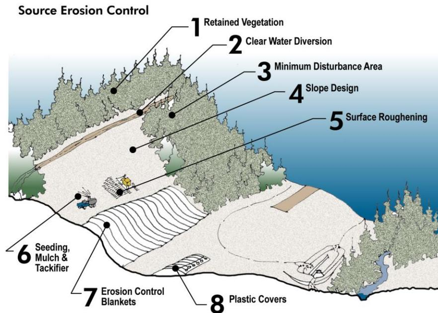
Figure 7.2: Source Control Measures to Prevent Erosion
