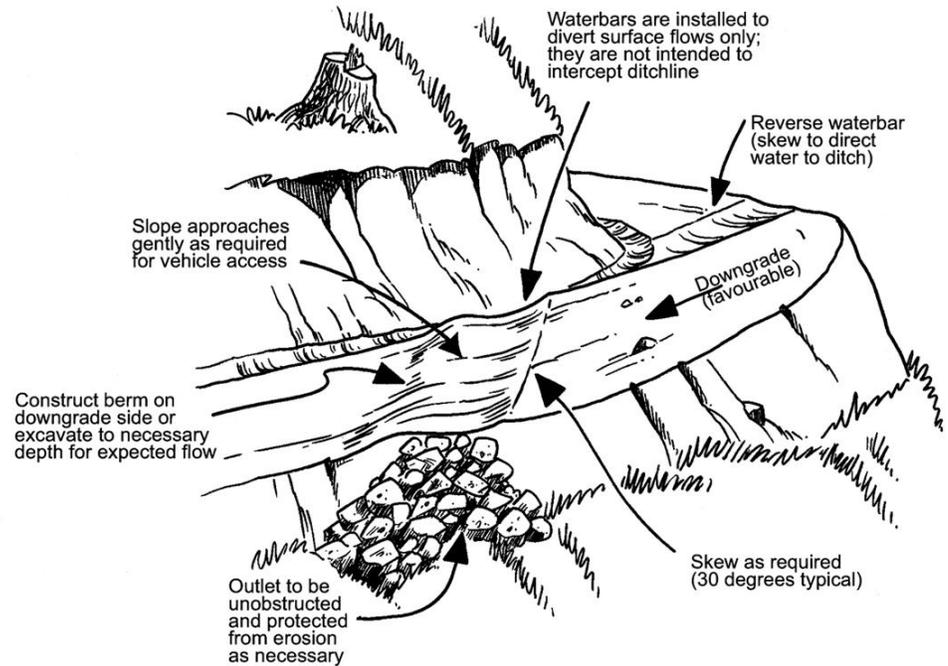
Figure 10.1: Water Bar Installation (from BC MOF, 2002)
