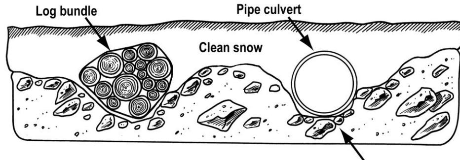
Temporary winter stream crossings using compacted snowfills. Culvert, heavy steel pipe, or log bundles allow meltwater to pass during warm weather trends.
