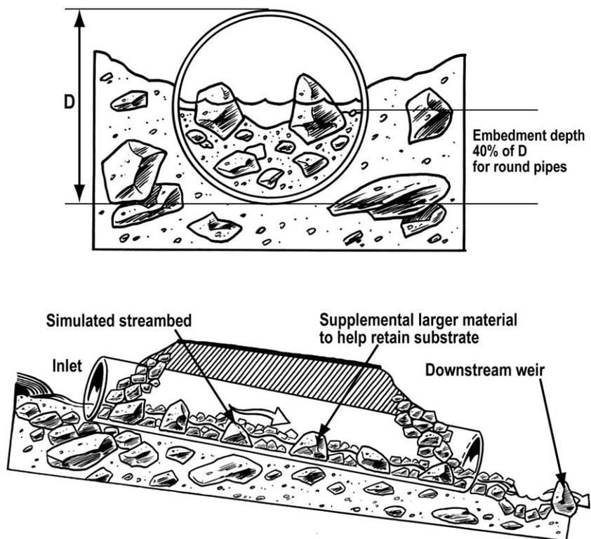
**Figure 10.8: Culvert/Streambed Cross-section and Profile**
