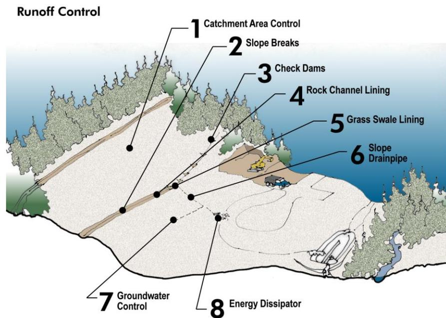
Figure 7.3: Surface Runoff Control
